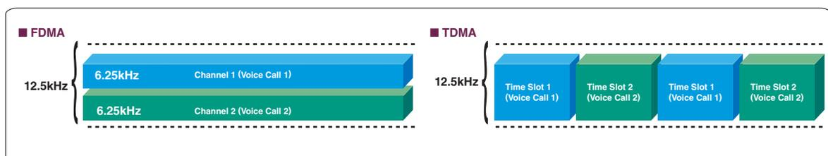
In TDMA, the same principle applies regarding bandwidth and frequency, but the signal is divided into time slots that allow the channel to have 'extra' capacity in the same bandwidth E.g. Two 6.25kHz 'equivalent' channels in a 12.5kHz channel. See the diagram below for a graphical explanation.
